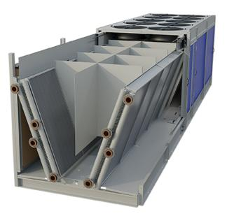
Equipping a unit with partition panels provides an **individual air intake duct for each and every fan** on the adiabatic condenser. This guarantees a higher capacity in case of fan failure by avoiding unintended air flows through an idle fan which bypasses the coil.
