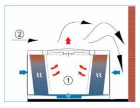
Incorrect Orientation of Tower and Neighbouring Walls 1. Induced Draft Cooling tower; 2. Prevailing Wind
