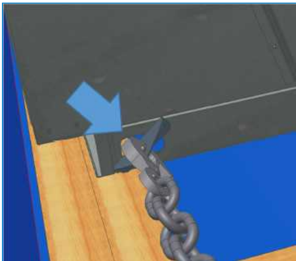
Remove unit out of container
